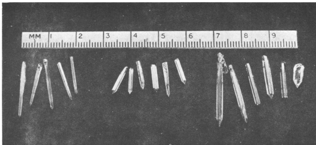
Figure 5 General view of crystals grown at increasing temperatures; from left to right: 1270, 1295, 1325° C.
